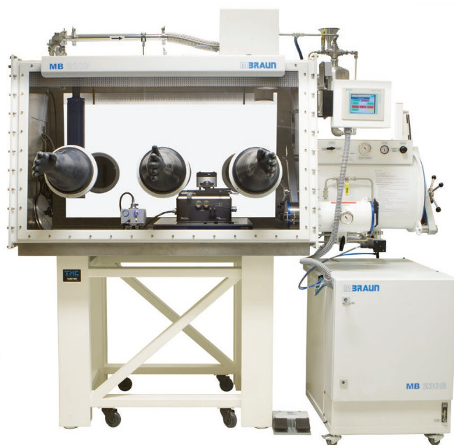
MFP-3D AFM in MB200 glovebox shown with air temperature and humidity control option. The images to the left were made with the MFP-3D in a glovebox.
