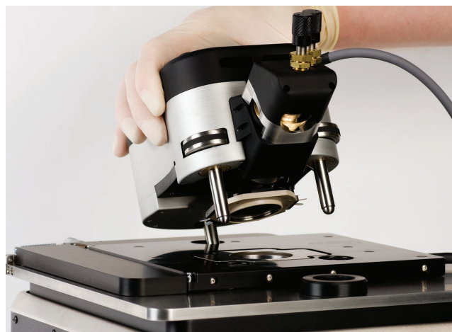
Closed Fluid Cell mounted to the cantilever holder on the MFP-3D head as it is being lowered into scanning position.
