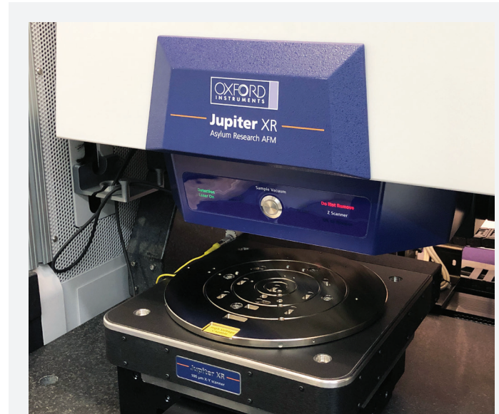
Jupiter XR AFM set up with the HVA150 accessory. All the components are automatically detected by the software for ease of setup and safety.
