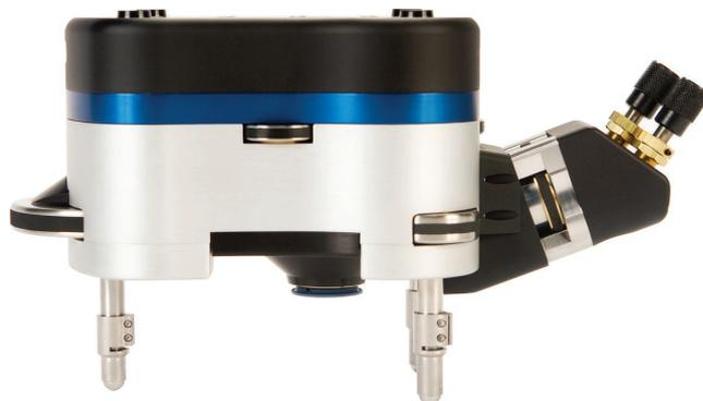
*The 40  $\mu\text{m}$  Z scan range Extended Head is ideal for imaging bioscience samples such as living cells, plant imaging, and pulling on long-chained molecules.*
