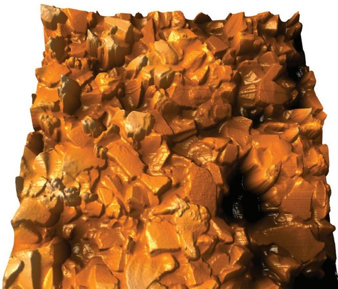
*2500 Grit Sand Paper. This sample required 19  $\mu\text{m}$  of Z range, 90  $\mu\text{m}$  scan.*
