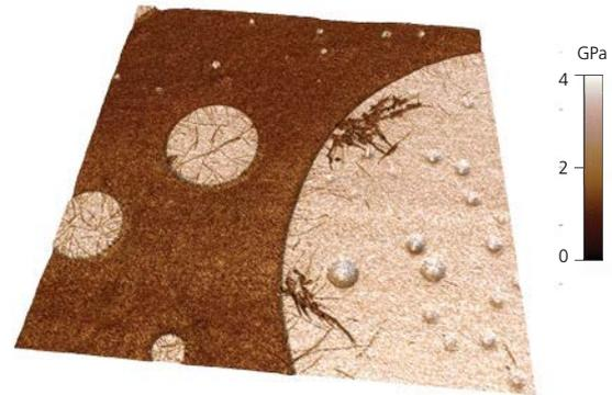
**Figure 3:** Polystyrene-polypropylene polymer blend thin film imaged using Fast Force Mapping mode. Elastic modulus is shown on 3D topography, 6 μm scan.
