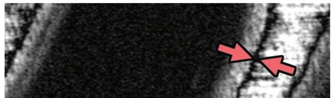
*Here, sMIM demonstrates a feature in the SRAM sample that measures 30.5 nm in width.*
