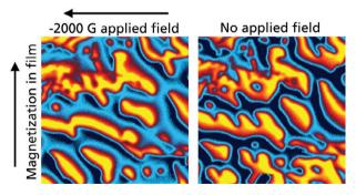
**Figure 4: Effect of in-plane field on Terfenol-D film** MFM phase images of the Terfenol-D disk, 10 µm scans. (left) Imaged while under a -2000 G field, and (right) after field removal. Image courtesy of S. Xie, Xiangtan Univ. and J. Li, Univ. Washington.
