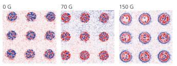
**Figure 6: Magnetic skyrmions in Co-based thin film pads** Imaged with MFM under out-of-plane magnetic fields. Each pad is ~900 nm in diameter. Images courtesy of K. Bouzehouane, Unité Mixte de Physique CNRS, Thales, Univ. Paris-Sud, Université Paris-Saclay, France.
