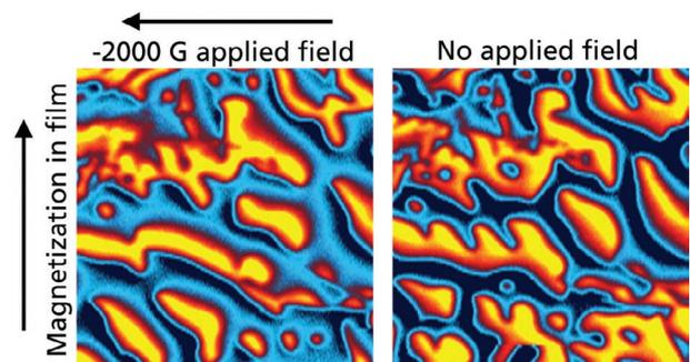
**Figure 4: Effect of in-plane field on Terfenol-D film**
