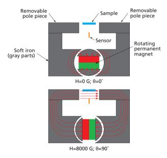
**Figure 2: Schematic of in-plane field configuration** The strength and sign of the magnetic field applied to the sample depends on the rotation angle ( $\theta$ ) of the rare earth magnet. At 0° or 180°, the magnetic flux is shunted away from the sample by the soft iron armature and pole pieces. As the magnet rotates, more and more flux is coupled instead through the sample. At 90°, the field is maximized.
